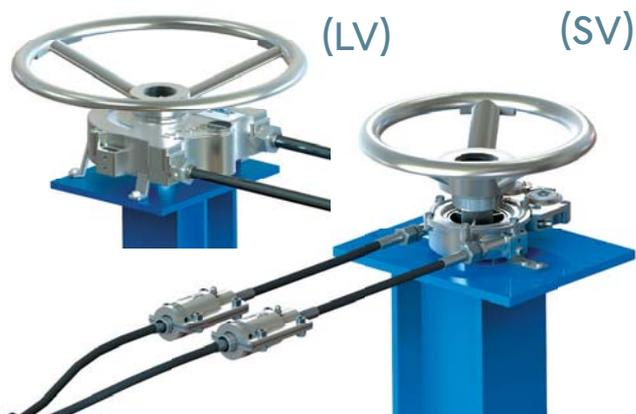
Operator stations are available in a variety of different gear ratios, providing a wide range of torque capabilities. A helically wound steel cable has a pitch the same as that of the cable gear. The precision gear-cable interface provides a positive force to the helix cable, which travels through the flexible conduit to the valve station actuator.
